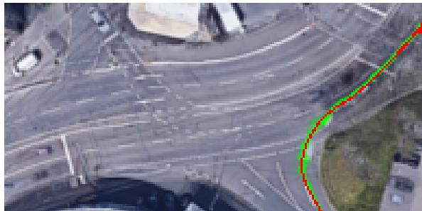
Fig. 6: Training results. Path planned by network (green) vs. human paths (red). Image data from Google Maps [17]
